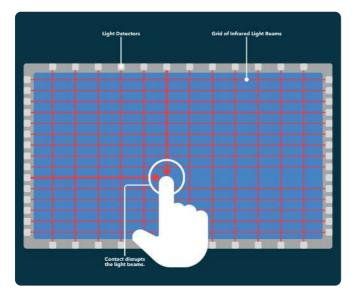
Infrared touchscreens use an array of infrared light-emitting diodes (LEDs) and photodetectors placed around the screen's edges. When an interrupts the obiect light beams between the LEDs and detectors, the system can pinpoint the touch location. This technology is highly durable and allows for the use of any object to interact with the
