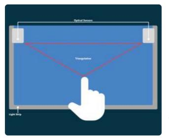
Optical touchscreens employ cameras and light sources to detect touch by interpreting the changes in light patterns on the screen surface. This technology allows for a highly responsive experience and can support multiple touch points simultaneously. Optical touchscreens are often used in large displays and interactive
