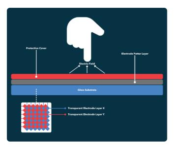
Capacitive touchscreens operate on the principle of electrical charge. They consist of a glass panel coated with a transparent conductor, typically indium tin oxide. When a finger touches the screen, it alters the local electrostatic field, allowing the system to detect the touch location. This technology provides superior clarity and supports multi-touch gestures,
