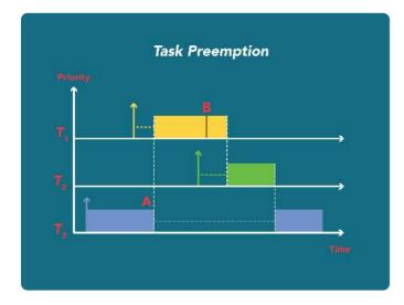
effective strategy for One minimizing task preemption time is to prioritize interrupts based on their criticality and categorizing urgency. By interrupts into different levels of importance, embedded engineers can assign appropriate priorities to ensure that high-priority interrupts are handled quickly and efficiently.
