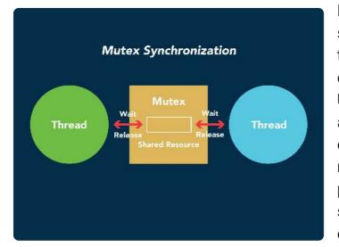
Mutexes another are synchronization mechanism that can be used to protect critical sections of code. Unlike semaphores, mutexes are used to ensure that only one task can access а resource at a time. This is particularly useful in scenarios where tasks need exclusive access to а
