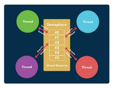
protect critical sections of code that must be executed atomically. By properly implementing semaphores, embedded engineers can ensure that interrupt handlers and tasks do not interfere with each other, reducing overall interrupt latency.
